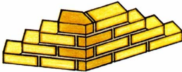
External angle using squint bricks
